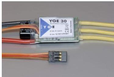
Fuente: Tomado de YGE 18 and 30A electronic speed controller (ESC).
