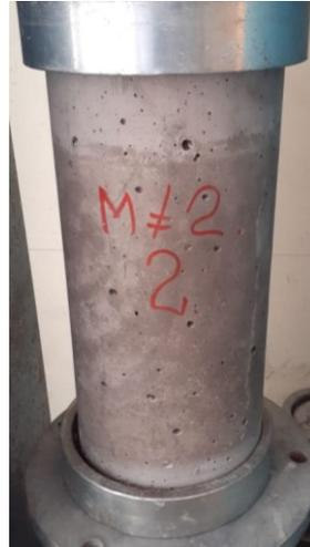
A cylindrical concrete specimen, 7 days old, marked with red ink as "M#2 2". It is mounted in a metal testing fixture and shows a smooth, uncracked surface.   |
