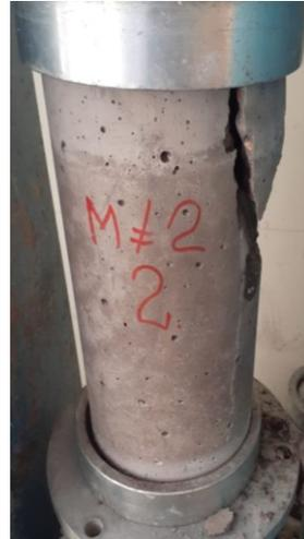
The same specimen after a compression test. It shows vertical cracking and some surface spalling, but the overall structure remains more intact than specimen 1.    |
