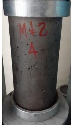
A cylindrical concrete specimen, 14 days old, marked with red ink as "M#2 4". It is mounted in a metal testing fixture and shows a smooth, uncracked surface. |
