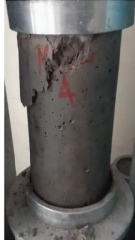
The same specimen after a compression test. It shows significant vertical cracking and a large portion of the concrete has been crushed and spalled at the bottom. |
